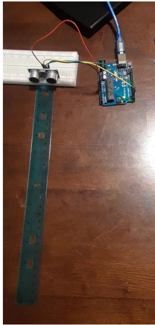
Figure 33: Testing the ultrasonic position sensors accuracy
