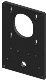
Figure 18: Stepper Motor Holder Plate Design. Reprint Confirmed from Open Builds [100]
